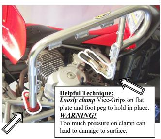
**INSTALL THE RIGHT SIDE NERF BAR** – Repeat Steps from Left Side Nerf Installation.
