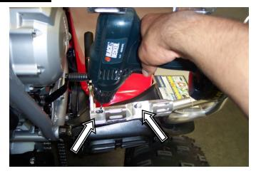
Bit. After Drilling Holes, Secure the Flat Plates to the Foot Pegs using the 6mm Flange Bolts, 6mm Flat Washers & 6mm Nylock Nuts supplied.
